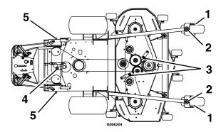
Number 4 (Idler Pivot (Pump Drive) Located Under Engine Deck
